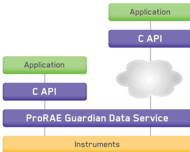
ProRAE Guardian SDK integrates real-time data from ProRAE Guardian with external customized applications and networks using the C API.
