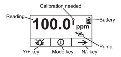
**Reading** Concentration of gas as measured by the
