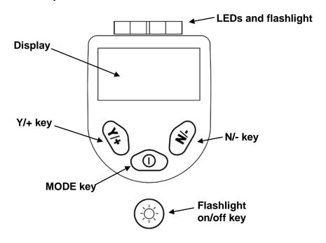
In addition to their labeled functions, the keys labeled Y/+, MODE, and N/- act as "soft keys" that control different parameters and make different selections within the instrument's menus. From menu to
