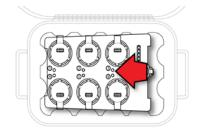
If batteries are already installed and require replacement, remove them. Then install new ones, being careful to match the batteries' direction to the polarities indicated by "+" in the battery holders.
