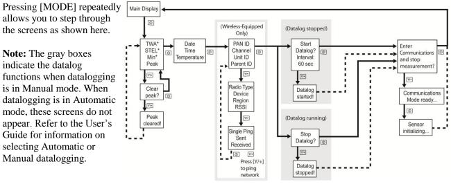
\* If your ToxiRAE Pro is configured with an oxygen (O<sub>2</sub>) sensor, TWA and STEL are not included in the menus because neither TWA nor STEL are calculated for this sensor. Min (for minimum) is included only when an oxygen sensor is used.
