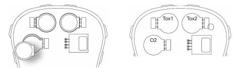
The LEL sensor is square and has four pins that insert into four plated holes in the PC board. When removing or installing an LEL sensor, lift it straight out and be careful not to bend the pins.
