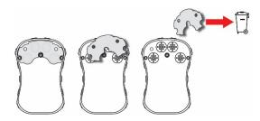
6. Set a new waterproof membrane filter on a flat surface. Peel off and discard one side's paper covering that protects the adhesive.
