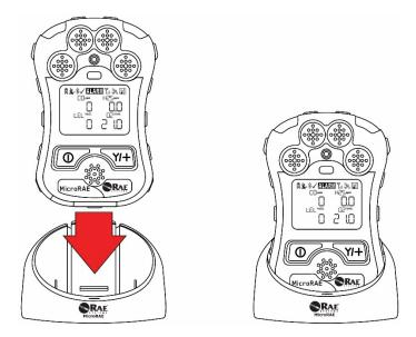
Remove the instrument from the cradle by tilting the release on the rear of the charging cradle away from the instrument and lifting the MicroRAE.
